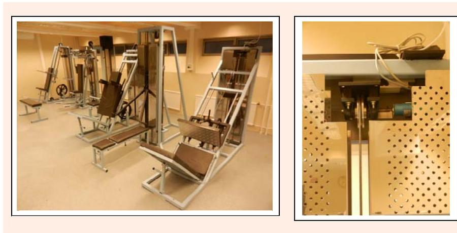
**Figure 3.** Sensor-equipped weight training machines and attached force (load cell) and way (rotary encoder) sensors to a leg press machine.
