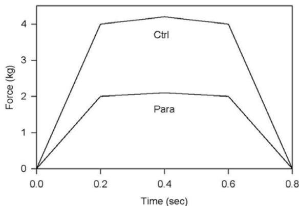
**Figure 5** Example of identical  $\frac{1}{2}$  RT and TPT in paralyzed and control muscle. Note the slower rate of  $\frac{1}{2}$  RT and TPT in paralyzed muscle because of lower force production in paralyzed muscle.
