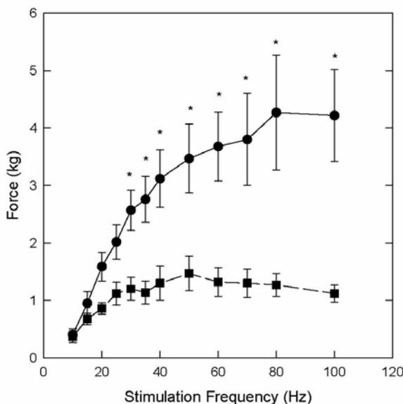
**Figure 1.** Force-frequency relationship measured in absolute force of TA in SCI (■) and control subjects (●). \* Significant difference between groups ( $p < 0.05$ ). (Error bars represent SE).
