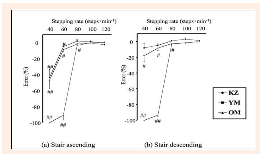
**Figure 1.** Pedometer accuracy during stair ascending and descending. Two illustrations show pedometer accuracy during stair ascending (a) and descending (b), respectively.
