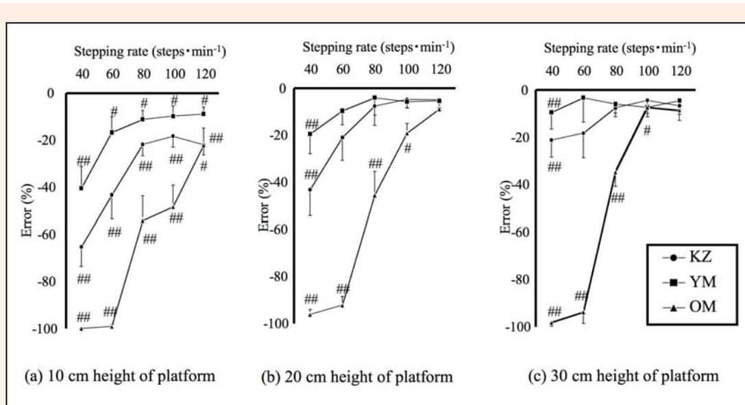
**Figure 2. Pedometer accuracy during bench stepping.** Three illustrations show pedometer accuracy during a bench stepping exercise by means of platforms that are 10 cm (a), 20 cm (b) and 30 cm (c) high, respectively.
