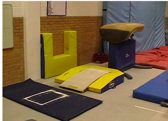
**Figure 2.** A photograph showing the vaulting area; the 'Sting' mat is the thin, blue mat in front of the spring board. The force platform was located directly under the 'Sting' mat, indicated by the white rectangle in the center of the 'Sting' mat.
