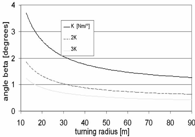
**Figure 6.** Torsion angle  $\beta$  function of turning radius (and for a given value of the skier velocity), for different stiffness values  $K$  of the ski-boot sole.
