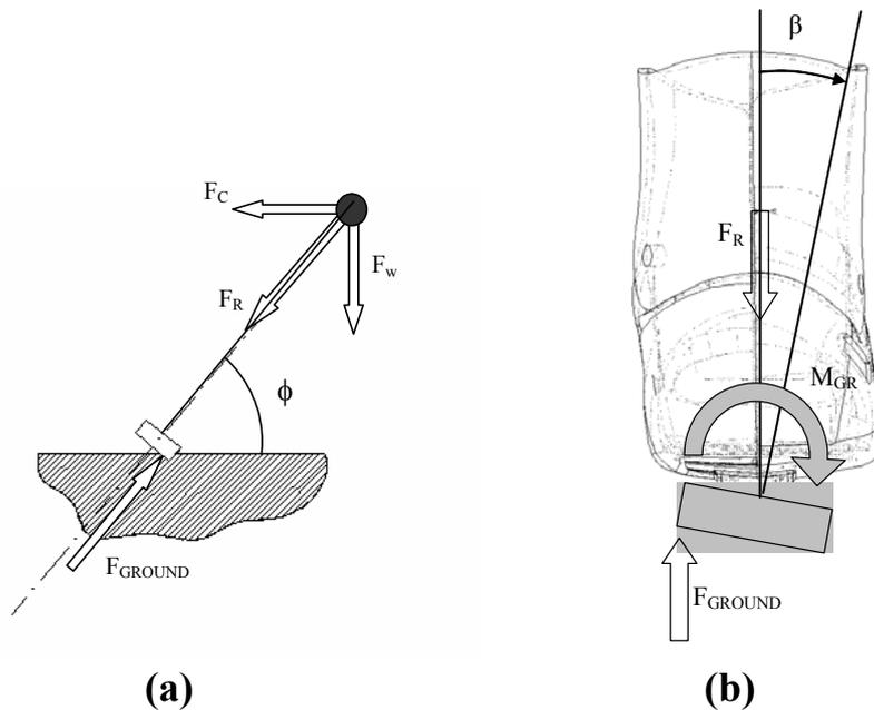
**Figure 2.** Forces acting on the skier during turning phase (a).  $F_{GROUND}$  (ground reaction) acts eccentrically respect to the skier axis generating  $M_{GR}$  (moment) that deforms in particular the lower part of the ski-boot (b).  $M_{GR}$  (moment) acting on the ski-boot sole causes sole and sole joint deformation resulting in drift angle  $\beta$  that reduces the real value of the ski inclination on the ground (b).
