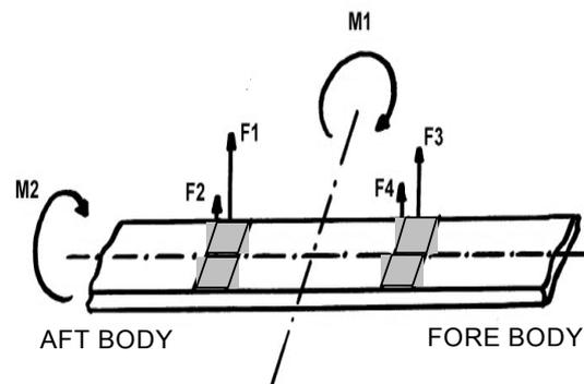
**Figure 4.**  $F_i$  represent load cells reaction forces that are acquired by the load cells monoaxially in the vertical direction. Only compressive loads are acquired, been considered positive. Using the 4 forces  $F_i$  it is possible to obtain momentum exerted along medio-lateral ( $M_1$ ) and antero-posterior ( $M_2$ ) axes. The total number of load cells used is 8, 4 for each ski.
