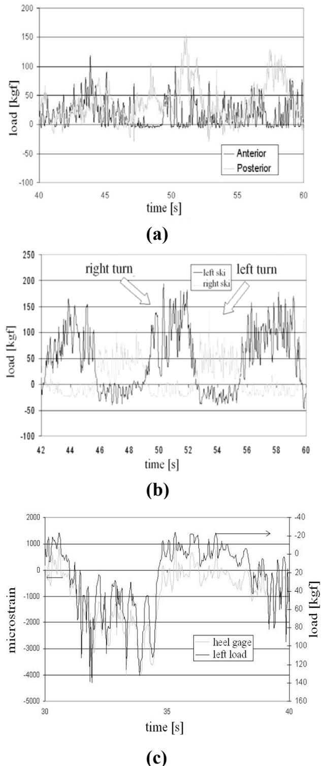
**Figure 5.** (a) Load signals F3 (anterior or shovel versus time) in black, and load signals F1 (posterior or heel versus time) in grey, as reported in Figure 4b, relative to the medial compartment of the same ski. (b) Load signals F1 (as reported in Figure 4b) for left and right ski (medial for one and lateral for the other). (c) Medially acting load on the left ski-boot and corresponding heel region deformation.
