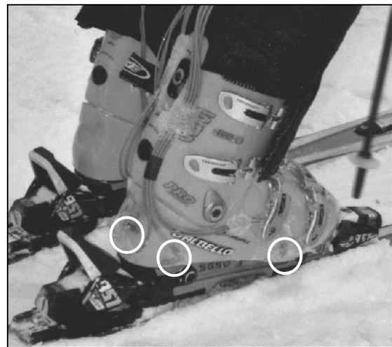
**Figure 3.** Ski-boots equipped with load cells and strain gages on the ski slope. Some strain gages locations are highlighted by white circles.
