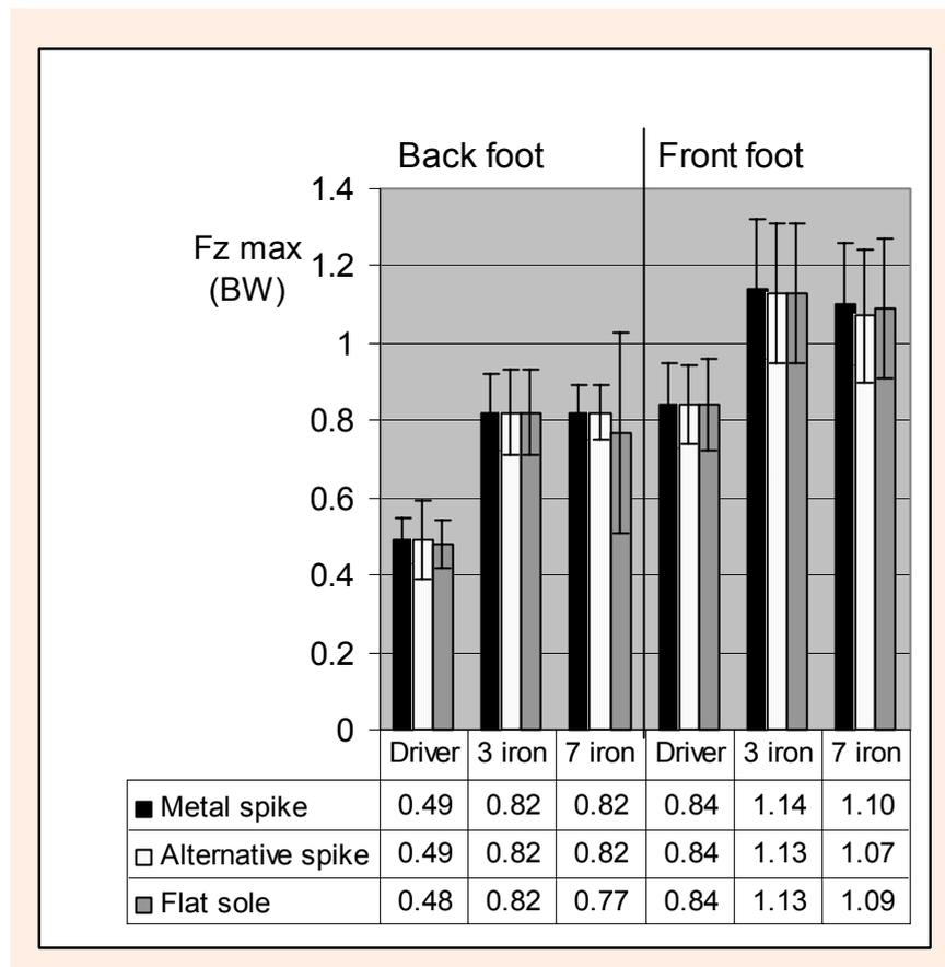
**Figure 4.** Mean maximum vertical forces ( $F_z$  max) generated at the back and front foot when wearing a traditional metal spike golf shoe, an alternative spike golf shoe and a flat sole shoe with no additional traction.
