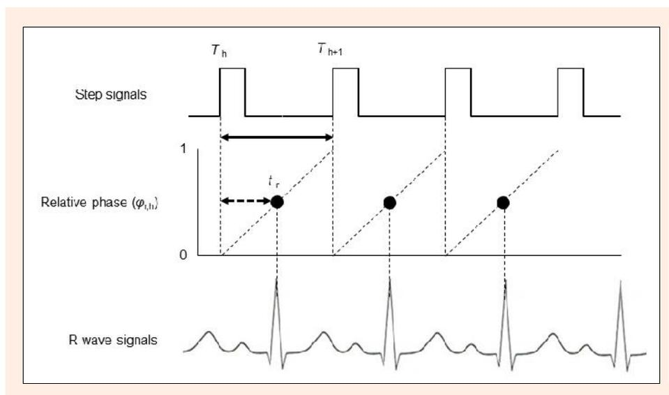
**Figure 1.** The computational theory used to calculate the relative phase relationship between the heartbeat and locomotor activity rhythms ( $\phi_{r,h}$ ). The square waves are step signals. Elevation of the wave indicates heel contact. The waves at the bottom of the panel are electrocardiogram signals. The sharply elevated wave is the R wave.
