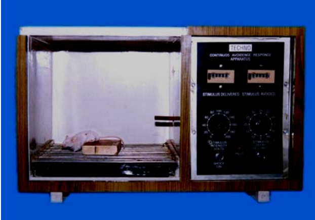
Picture 3. Passive avoidance apparatus.
