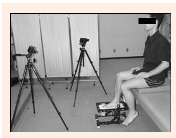
Figure 1. 3D ankle position analysis system. Measurements system using two digital cameras and a platform that allows dorsiflexion, palantarfexion and inversion of the ankle.
