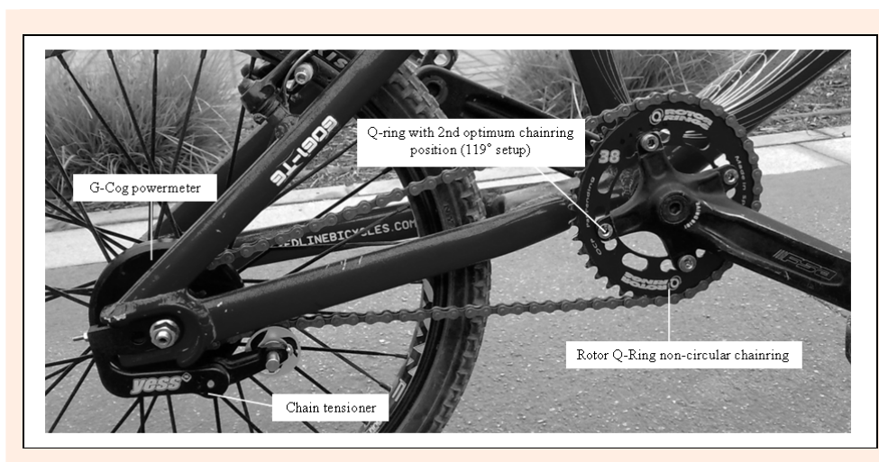
Figure 3. The customized BMX bicycle showing the non-circular chaining in 2 nd optimum chaining position or 119°, Yesspro chain tensioner and G-Cog electronic measuring device.
