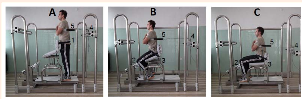
Figure 1. Measurement setup for trunk flexion isometric strength testing in standing (A), kneeling (B) and sitting (C) body position. A multi-purpose dynamometer enables measurements in sagittal, frontal and transverse planes. The strap across the pelvis (1) and the knee support bar (2) provide good segmental stability. The height, inclination and horizontal position of the seat (3) could be regulated manually according to subjects' morphological characteristics. Lateral bars with force sensors (4) could be moved vertically and fixed at the appropriate height. A rigid rope connects the belt (at mid sternum level) (5) with the force sensor.
