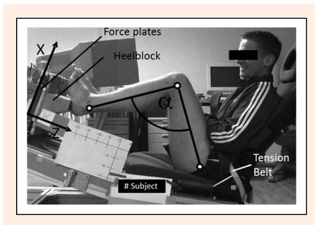
**Figure 1.** Exemplary positioning of the participants on the negatively inclined isometric leg-press slide.
