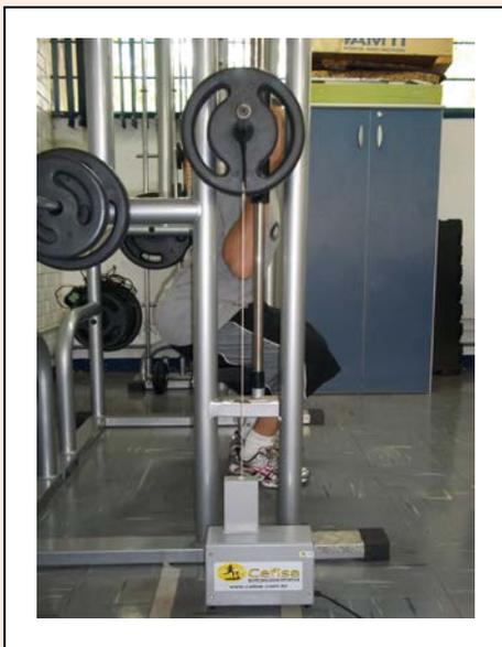
**Figure 2.** Power produced during squat exercise was measured by a linear position transducer attached to the barbell. Subject was instructed to perform the concentric phase as fast as possible.
