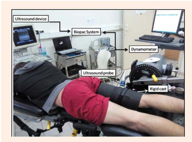
**Figure 1.** Example images from the experimental set up. After the injury location was identified, the probe was stabilized and secured with a customized rigid cast. The dynamometer and ultrasound data were fed to a Biopac unit for simultaneous display of their all data (Please note that participant is not secured on the dynamometer chair for illustration purposes).
