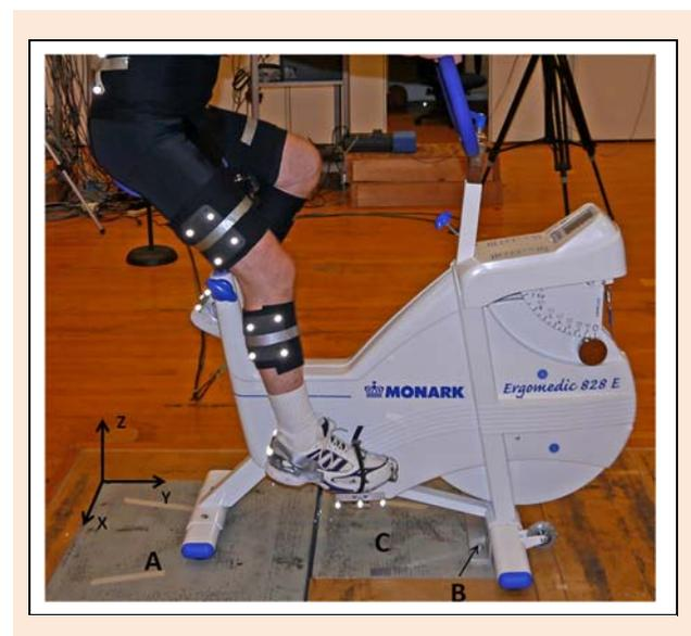
**Figure 1.** The stationary cycle ergometer setup and marker placements on the pedal and lower limb. The instrumented pedal is on the left side.
