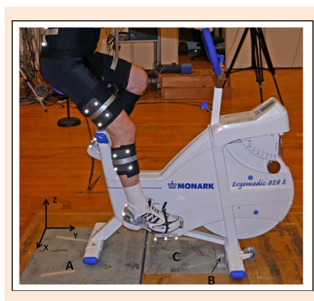
Figure 1. The stationary cycle ergometer setup and marker placements on the pedal and lower limb. The instrumented pedal is on the left side.
