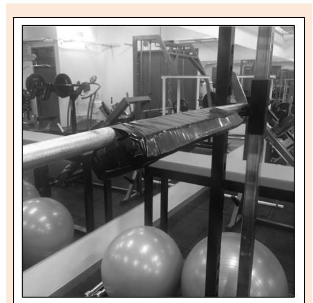
Figure 2. The rubber padding designed to mimic the density of skeletal muscle tissue affixed to a metallic impact surface used in the impact induced muscle damage (IIMD) collision simulator.
