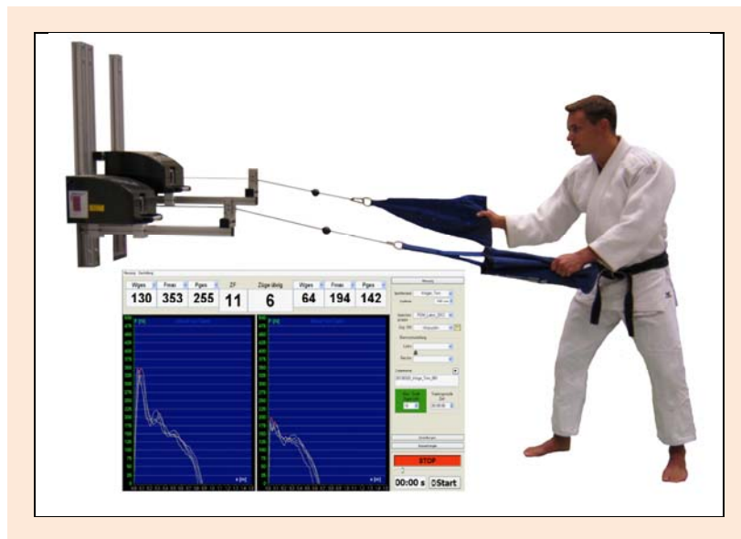
Figure 3. Judo ergometer (JERGo ® ) system with real time display for judo-specific performances (i.e., mechanical work, maximal force, power) and force displacement characteristics for the pulling (left display) and the lifting (right display) arm during repeated kuzushi movements.
