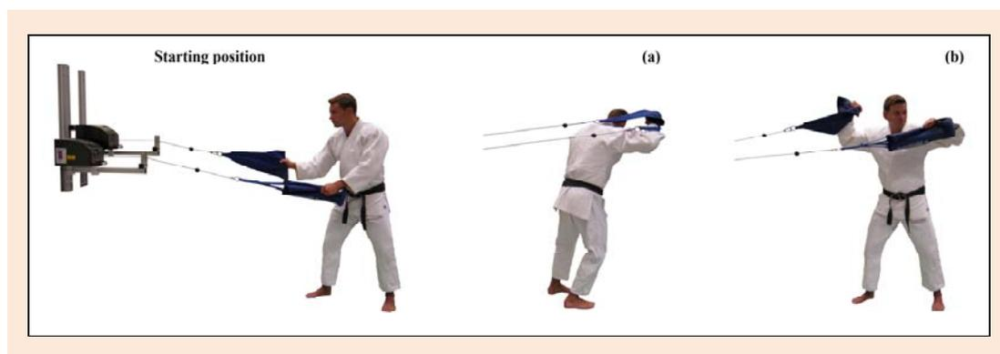
**Figure 1.** Setup for the assessment of (a) *kuzushi with tsukuri* and (b) *kuzushi without tsukuri* at the judo ergometer (JERGo<sup>®</sup>) system.
