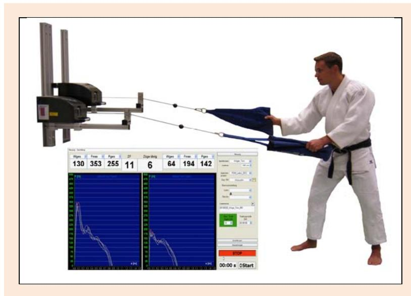
**Figure 3.** Judo ergometer (JERGo<sup>®</sup>) system with real time display for judo-specific performances (i.e., mechanical work, maximal force, power) and force displacement characteristics for the pulling (left display) and the lifting (right display) arm during repeated *kuzushi* movements.
