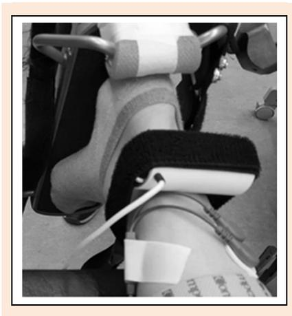
**Figure 2.** The set-up for the local vibration device with the electromyography on the shank. The foot was attached to the isokinetic device.
