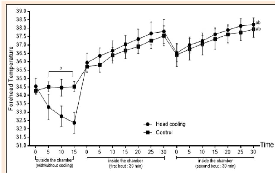
**Figure 2. Forehead temperature ( $^\circ\text{C}$ ) of participants in experimental trials.** Mean forehead temperature was lowered in HC trial than CON trial during the precooling session ( $n=10$ ). “a” indicates a significant main effect for time for both trials ( $p < 0.001$ ). “b” indicates large effect size (HC  $d = 8.41$ , 7.1, CON  $d = 10.38$ ) for both trials over time. “c” indicates a large effect size between trials during cooling ( $d = 2.12 - 4.4$ ).
