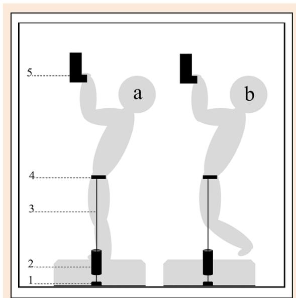
**Figure 2.** Schematic presentation of the test set-up during the isometric pull-up showing 1) expansion bolt in the concrete floor, 2) the force cell, 3) the static daisy chain, 4) the climbing harness, and 5) the 23 mm rung. The gray figure represents the climber before (a) and while (b) exerting maximal force. No horizontal or vertical displacement occurs between the two images.
