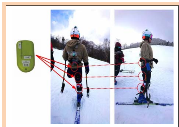
Figure 1. The locations of the inertial measurement units on the athlete's body segments (pelvis, right thigh, and right shank).
