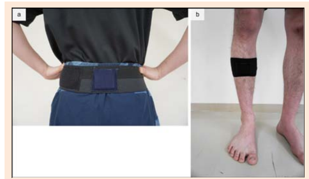
Figure 1. Location of the inertial sensors on the sacrum (a) and shank (b).
